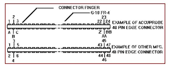
To avoid confusion for the probe card assembly or maintenance personnel, an edge connector translation table should be constructed to avoid mis-wiring of the card assembly. An example is shown below.
