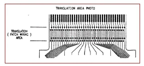
The principle objective of a probe card is to properly connect a test pad to a probe through the printed circuit traces to the edge connector, which interfaces with the tester. A particular test pad ultimately connects to one port of the tester, which is sometimes referred to as a scanner.
